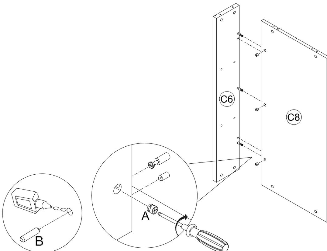
Step 3: Attach the Front Support Panel(C5) and Support Panel(C6) and Back Pane(C8) and Bottom Support Pane(C9) to the Right side Panel(C3).Use a Phillips Head Screwdriver to turn the Cam Lock (A) to lock onto the head of Cam Pin(A).
