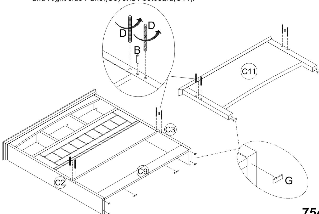
Step 9: Use a Wrench(I) to tighten the Side Rails(C10) to the Left side Panel(C2) and Right side Panel(C3) and Footboard(C11) with Bolt(D) and Cover(F).
