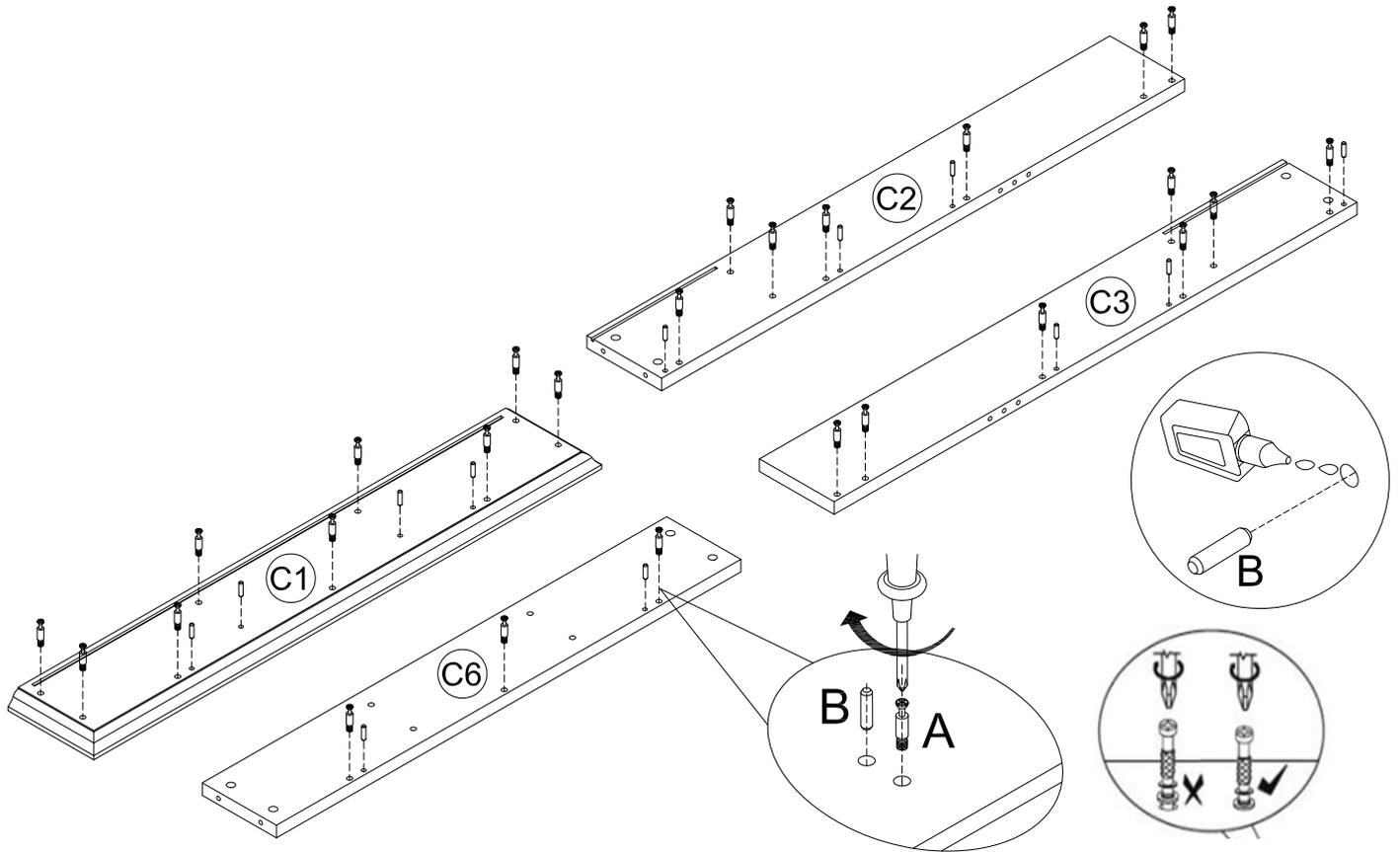
Step 2: Attach the Back Panel(C8) to the Support Panel(C6).Use a Phillips Head Screwdriver to turn the Cam Lock (A) to lock onto the head of Cam Pin(A).
