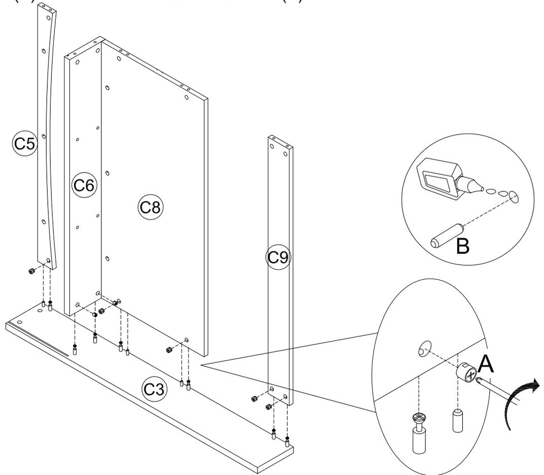
Step 4: Attach the Left side Panel(C2).Use a Phillips Head Screwdriver to turn the Cam Lock (A) to lock onto the head of Cam Pin(A).
